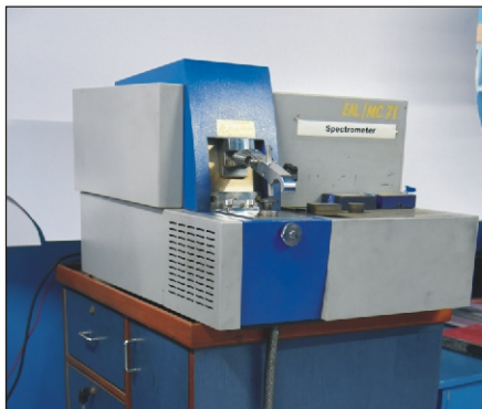
7 Metal Analyzer (SPECTROMAXx Germany)
