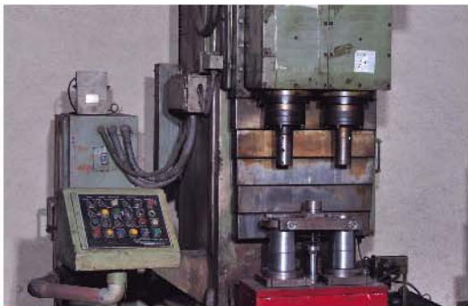
3 SPM for Vertical Final Boring
